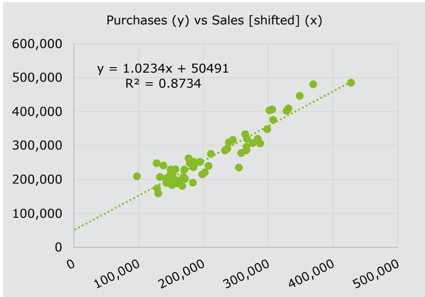
Apparent losses, such as meter error, scale with sales
